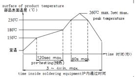
9 Automatic Flow Soldering (自动焊接)
