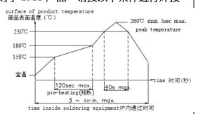
**Automatic Flow** 21 Soldering (自动焊接) Caution: the condition mentioned above is a temperature on the PWB surface on which parts are mounted. There are cases where PWB temperature greatly differs from switch's surface temperature depending on PWB material, size, thickness, etc. The switch's surface temperature shall not allowed to exceed 260°C
